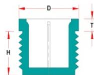
Special threaded plugs made of PA 6, designed for screwing radiators and heat exchangers. These are plugs with hidden threads. This range of plugs is specially designed for various types of heating elements.
